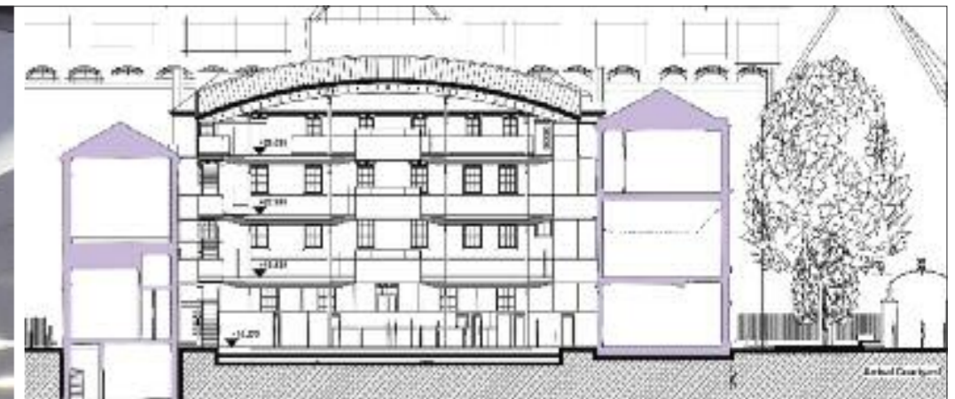
Cross section from the new gable end towards the original station hotel showing how the new floors and roof sit within the original structure, self-supported and connecting to the old building via bridge links.
